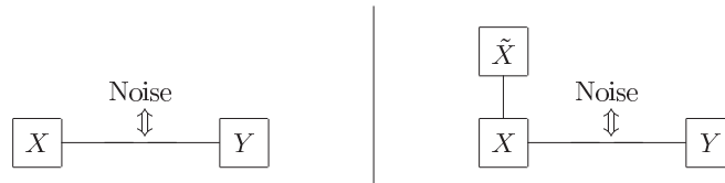
Figure 9.2. Given a Markov process X \rightarrow Y we may first make a copy of X , \tilde{X} , before subjecting X to the noise which turns it into Y .
