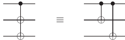
Figure 4.13. Controlled-NOT gate with multiple targets.
