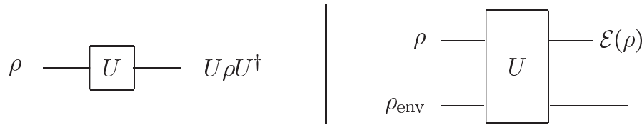
Figure 8.3. Models of closed (left) and open (right) quantum systems. An open quantum system consists of two parts, the principal system and an environment.
