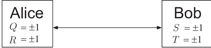
Figure 2.4. Schematic experimental setup for the Bell inequalities. Alice can choose to measure either Q or R , and Bob chooses to measure either S or T . They perform their measurements simultaneously. Alice and Bob are assumed to be far enough apart that performing a measurement on one system can not have any effect on the result of measurements on the other.
