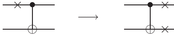
Figure 10.20. A controlled-NOT gate can cause an error to propagate so that instead of affecting one qubit, it affects two. This is also true when encoded qubits are used, and an encoded controlled-NOT is implemented, as discussed in the text.
