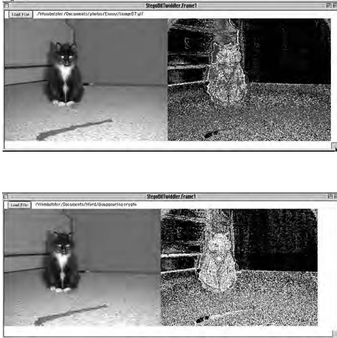
Figure 17.1 The top window shows a picture and its least significant bits before approximately 6000 bytes were hidden in the image with EzStego. The image had a capacity of 15,000 bytes. The bottom window shows the image and the least significant bits afterward.
